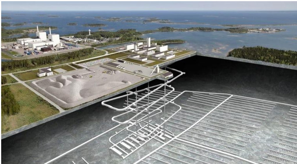
Figure 8 – Figure - SKB's Swedish deep geological disposal concept
